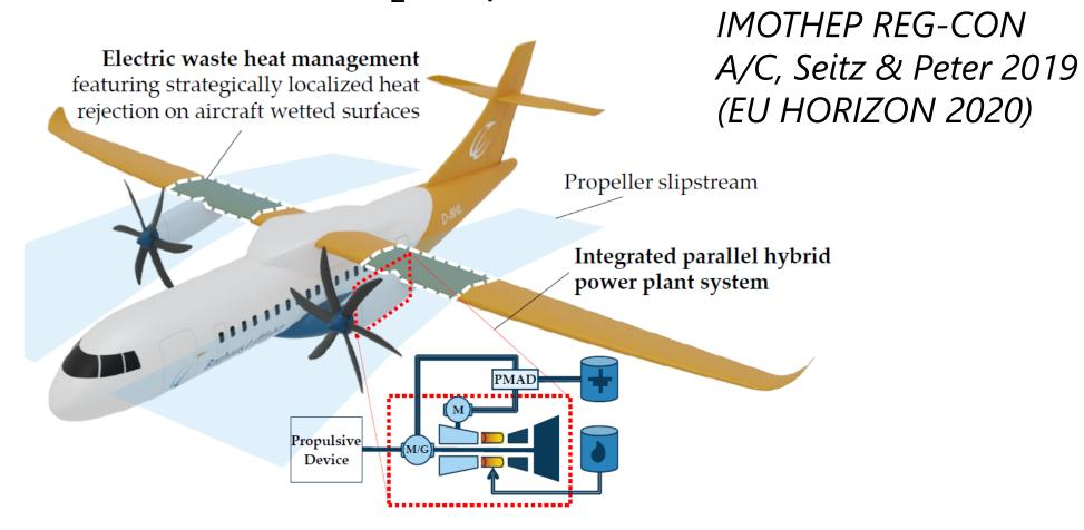
Surface-embedded heat exchangers have a high potential for an efficient rejection of head loads:
